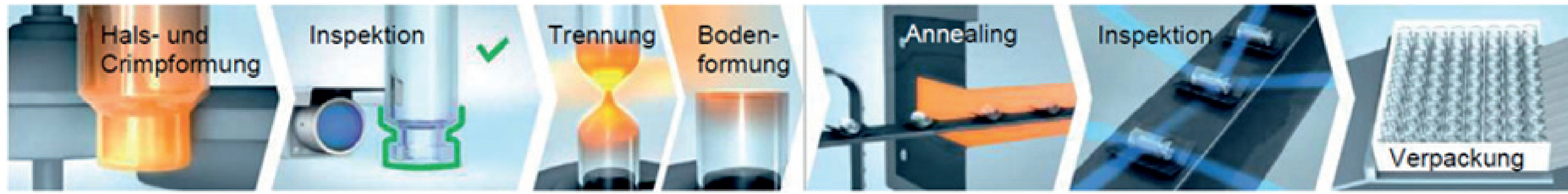
PROCESS STEPS FOR THE MANUFACTURE OF PHARMACEUTICAL VIALS MADE OF GLASS TUBES (SOURCE: SCHOTT AG)
